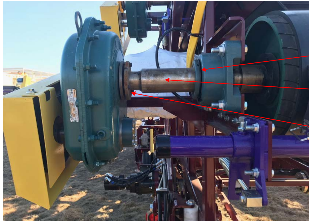
Typical Shaft/Bearing Installation at Drive Pulley
